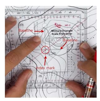
**Step 4:** Read the degree value at the intersection of your extended line with the protractor's degree scale. This reading represents your grid azimuth from point A to B in degrees.
