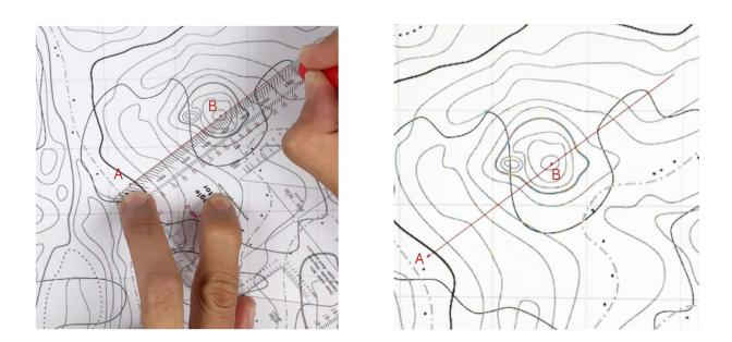
**Step 2:** Place the protractor's index mark where your line crosses a north-south **grid line** and align the protractor's baseline with the north-south grid line.
