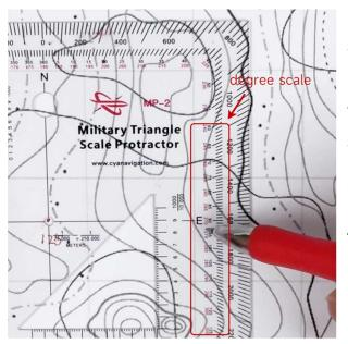
**Step 5:** Now, draw a straight line from the center hole to the degree mark along the protractor's edge. This line represents the azimuth you need to follow.
